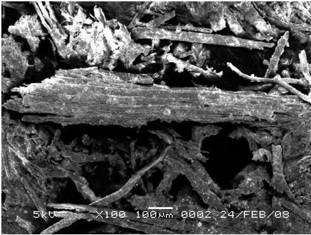
Fig. 3. SEM examination of the straw board
