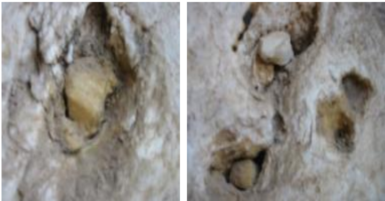
Figs 67-68 display the third type of vugs and open spaces is large 30-80 cm. long into which protrude almost spherical surface of the travertine of chapels at Karnak of Wadi El-Assiuty
