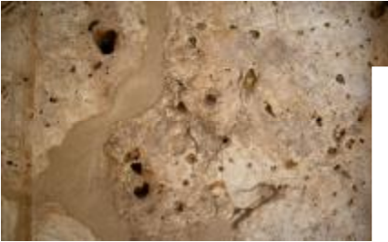
Figs 69 – 71 display the second type of vugs which is confined to parts which appear to the outer surfaces of the travertine of chapels at Karnak of Wadi El-Assiuty, of the alabaster deposit , the vugs occur elongated is of the milky white type
