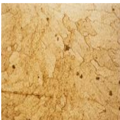
Figs. 1-5 Thin sections microphotograph of a an alabaster sample of Wadi El Assiuty the source of alabaster at Karnak displays drusy mosaic of calcite (disoriented small calcite crystals), the texture is an harmonic mixture of fibrous and equant mosaics resulting in the fine layering of the alabaster a variety of bands of variety of translucency degrees especially delicately banded which due to alternation of bands of translucent creamish type with the opaque milky white type , a yellowish translucent band consists of elongated fibrous crystals , the texture is a fibrous mosaic alternating with an equant mosaic , abundant amorphous carbonate either as patches or as bifurcating vein lets , and there is an important note : there no almost micro cracks or fissures with presence of some gypsum crystals comparing with the weathered samples were taken from Karnak according to explain forth coming .
