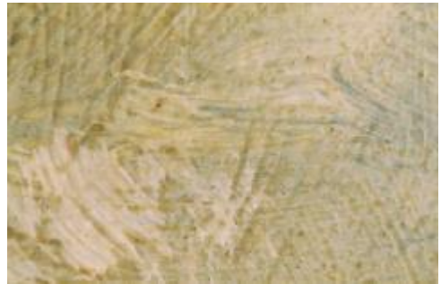
Fig.4 Thin paint layer was applied on top of artificial cracks.
