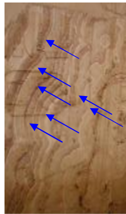
Figs. 55- 60 Display the Egyptian alabaster (Travertine) surfaces of chapels of Karnak of Wadi El-Assiuty characterized of presence of botryoidal or colloform structure and the planes of the colloform structure are weakness planes because of the tendency to break along these planes (arrows) , also display covering the convex and the outer surface of stone with a thin layer of red iron oxide and that indicts it belongs to The 3 rd type of the colloform structure forms which is of colloidal origin and existence of the spheroidal surfaces - which due to surface tension phenomena
