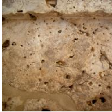
Figs 69 – 71 display the second type of vugs which is confined to parts which appear to the outer surfaces of the travertine of chapels at Karnak of Wadi El-Assiuty, of the alabaster deposit , the vugs occur elongated is of the milky white type
