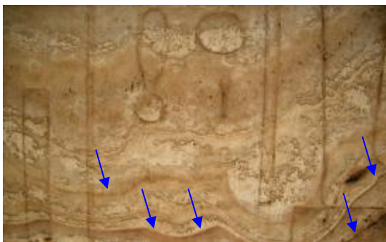
Figs. 55- 60 Display the Egyptian alabaster (Travertine) surfaces of chapels of Karnak of Wadi El-Assiuty characterized of presence of botryoidal or colloform structure and the planes of the colloform structure are weakness planes because of the tendency to break along these planes (arrows) , also display covering the convex and the outer surface of stone with a thin layer of red iron oxide and that indicts it belongs to The 3 rd type of the colloform structure forms which is of colloidal origin and existence of the spheroidal surfaces - which due to surface tension phenomena
