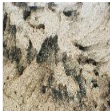
Figs. 1-5 Thin sections microphotograph of a an alabaster sample of Wadi El Assiuty the source of alabaster at Karnak displays drusy mosaic of calcite (disoriented small calcite crystals), the texture is an harmonic mixture of fibrous and equant mosaics resulting in the fine layering of the alabaster a variety of bands of variety of translucency degrees especially delicately banded which due to alternation of bands of translucent creamish type with the opaque milky white type , a yellowish translucent band consists of elongated fibrous crystals , the texture is a fibrous mosaic alternating with an equant mosaic , abundant amorphous carbonate either as patches or as bifurcating vein lets , and there is an important note : there no almost micro cracks or fissures with presence of some gypsum crystals comparing with the weathered samples were taken from Karnak according to explain forth coming .
