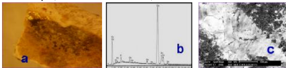
Fig. 16 Gilded sample (previous intervention) from Khankah and mausoleum of sultan Beybars El-Jashankir: a) Microphotography corresponding to the sample (deteriorated gilded); b) EDX analysis in surface layer of the sample shows its components; c) SEM micrograph of the sample (surface deterioration observed).
