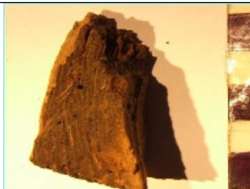
Fig.48- shows deteriorated wooden sample ( Pinus Leucodermis Ant. (Pinaceae) )
