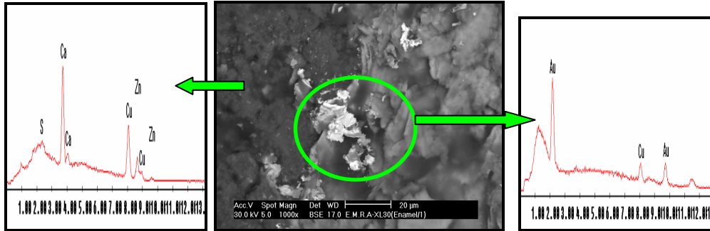
Fig. 4 SEM image and EDX analysis result of gold foil.
