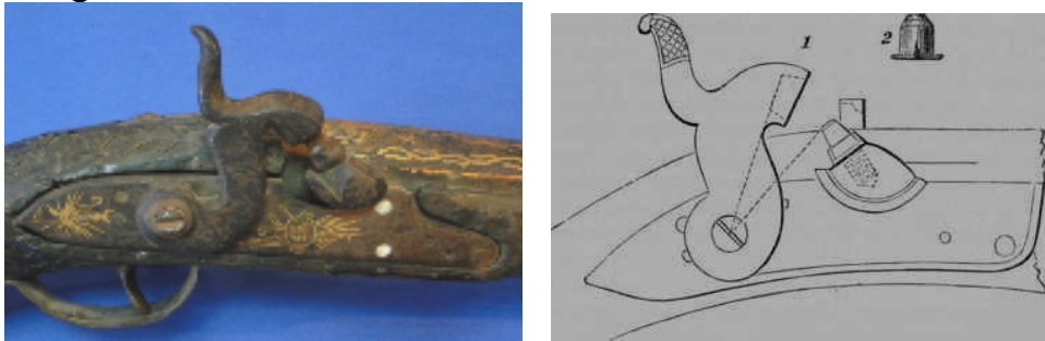
Fig (2a,b) a)details of percussion firing mechanism, b)1-hammer 2-percussion"cap"after Ripley, G.and Dana, C., 2
