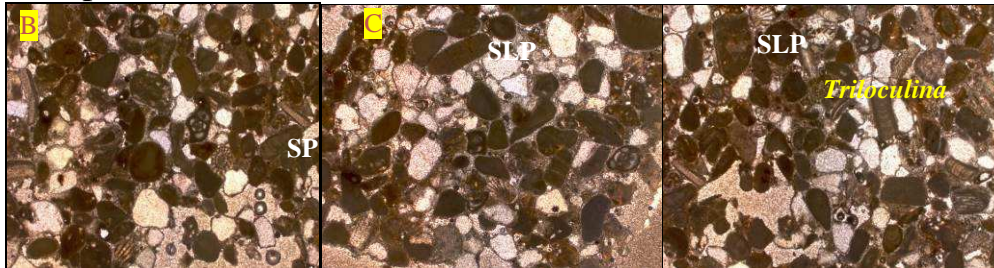
Fig. 5a-c Petrographic view of limestone sample (W2) shows the weathered stone heterogeneous pore system contains ferric oxides and hydroxides (black spots) and shows the components are fossil fragments, structural less Peloids (SLP), quartz grains, structure peloids (SP) and iron oxide (X25).
